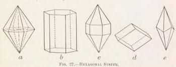
a, Hexagonal Pyramid showing axes; b, Prism; c, combination of Pyramid and Prism, without basal planes; d, Rhombohedron; e, Scalenohedron.
